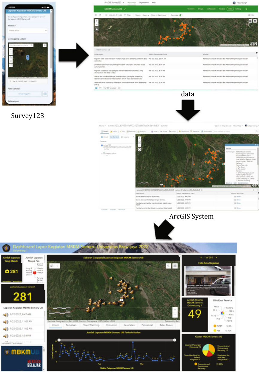
Fig. 34.16 Data integration and synchronisation between Survey123 and ArcGIS Dashboard. Source Created by Researchers, 2022
