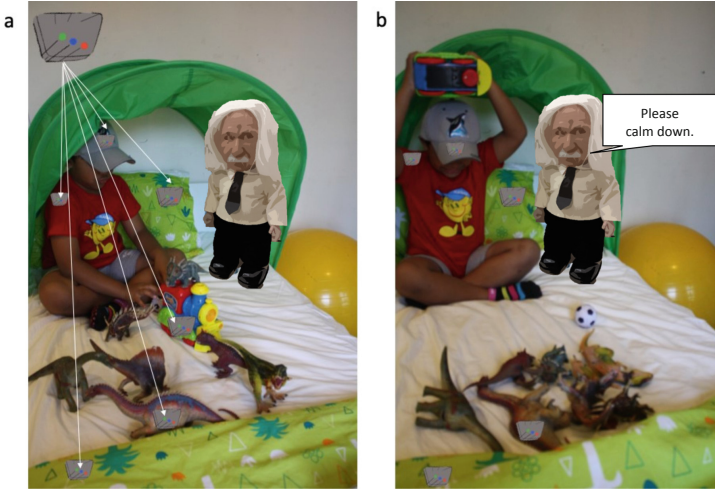
Fig. 4. A child displaying unwanted behaviors while interacting with his surrounding. (a) Possible locations of the Smart, Snap-on devices on the child's cap, shirt, pillow, blanket, and toys. (b) A social companion robot will say calm messages when the sensors detect aggressive behaviors.
