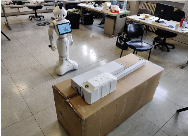
Fig. 3. Initial setup, with the robot ready in front of the structure with the Aruco markers. The two additional cameras on board the robot, as well as some of the markers hidden in the structure, can be seen in the picture. The operator is on the opposite side of the room, with the robot not on their line of sight.
