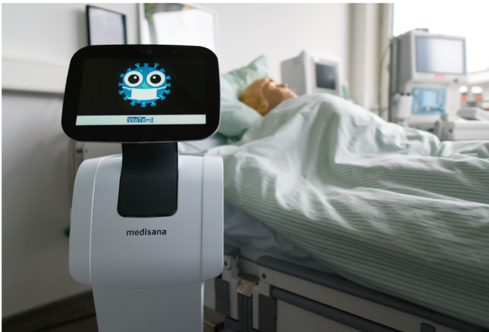
Fig. 1. The autonomously home care humanoid robot, called Temi, for establishing video telephony between patients and relatives via an online system during the virus outbreak, presented by Follmann et al. [9].
