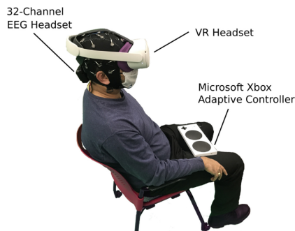
Fig. 3. Experiment Setup: One of the participants wearing 32-channel EEG headset, VR headset, and interacting with the Xbox Adaptive Controller
