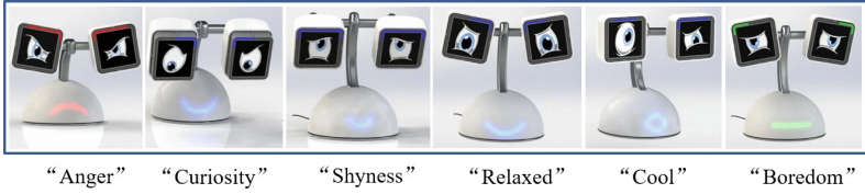
Fig. 3. Examples of a few Haru’s emotions expressed through the animated emotive routines.
