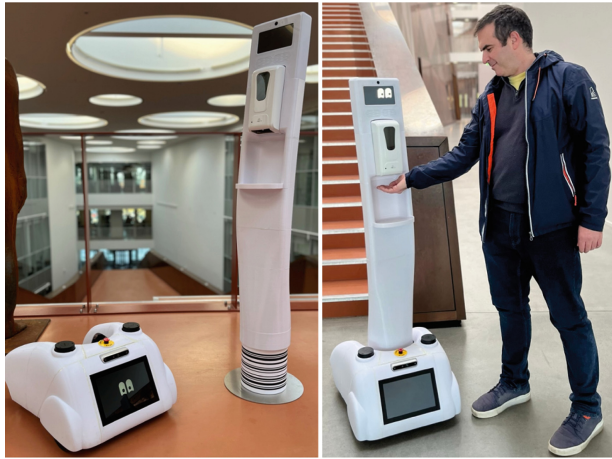
Fig. 1. The mobile base and the stand separated (left) and the unified hand disinfection robot in interaction with a person (right).
