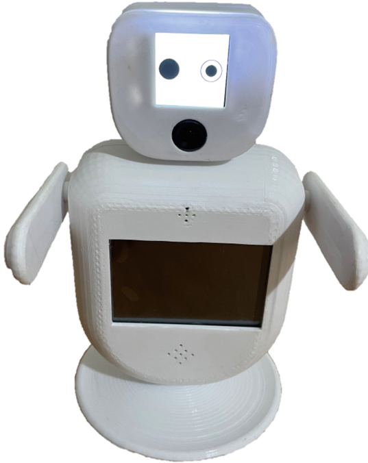
Fig. 1. The developed mini-humanoid robot that was considered in this study.
