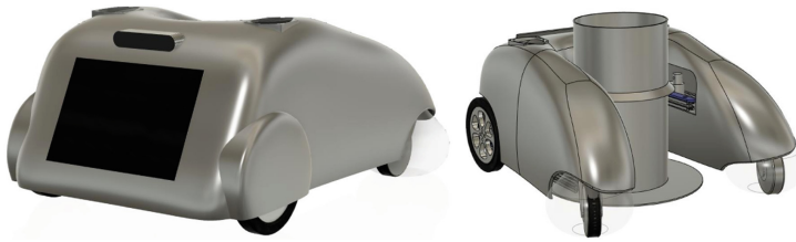
Fig. 2. A rendered view of a) the front of the mobile base and b) the back of it with a lower part of the disinfection stand attached.
