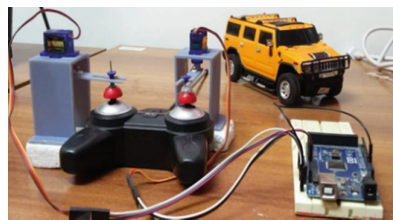
Fig. 2. Final joystick controller System
