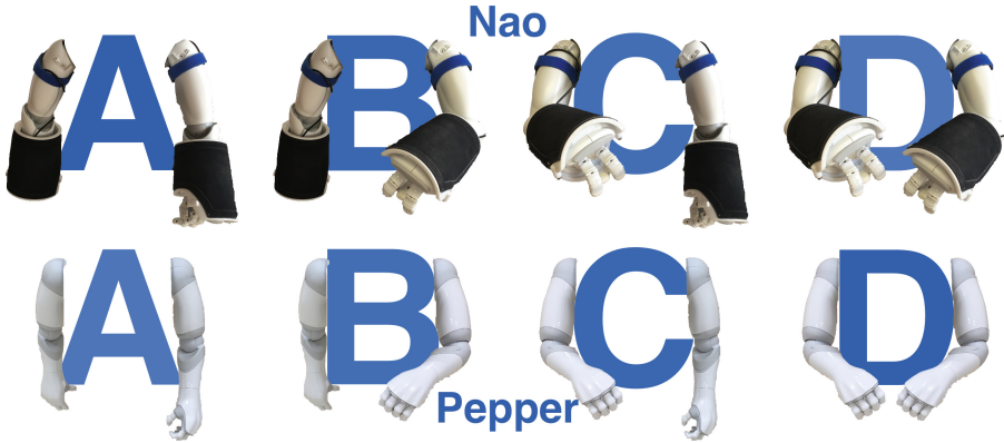
Fig. 3. Startle reactions – arm movements schematics. (Top) Nao, (Bottom) Pepper. (A) Touched hand back, other hand still. (B) Touched hand back, other hand forward. (C) Touched hand forward, other hand still. (D) Touched hand forward, other hand forward. See Figs. 1, 2 for complete robot photos.
