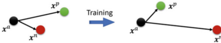
Fig. 7 Triplet loss: minimizes the distance between two similar class examples (anchor and positive) and maximizes the distance between two different class examples (anchor and negative)
