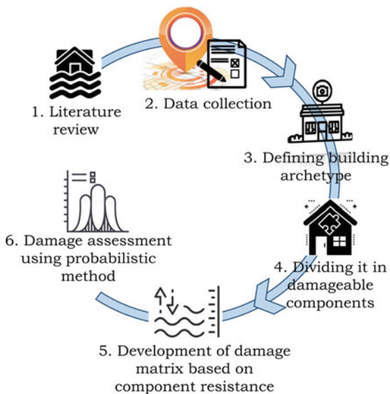
Fig. 8.4 Building damage assessment method
