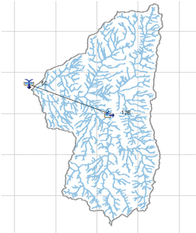
Fig. 1.4 The developed HEC-HMS model for the Petra watershed
