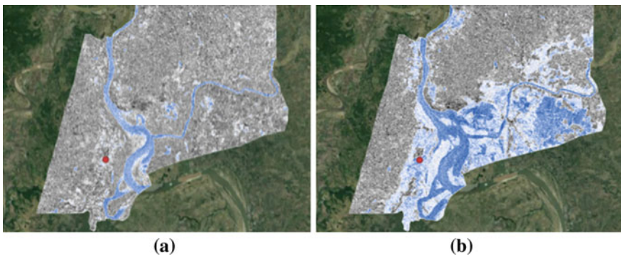
Fig. 4.10 Sentinel 1 data in Alcala, Cagayan a before, and b after Typhoon Ulysses (Vamco)
