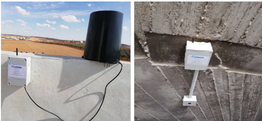
Fig. 1.2 Sample installations of the tipping bucket (left) and ultrasonic (right) sensors
