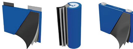
Fig. 3. Common forms of lithium ion cells; pouch (left), cylindrical (middle) and prismatic (right) (reproduced from Ref. [10] with permission from MDPI).
