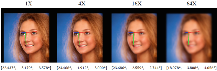
Fig. 7. Downsampling factor vs. the angles of yaw, pitch & roll. The ground-truth values are [19.495^\circ, 2.322^\circ, -4.536^\circ] .
