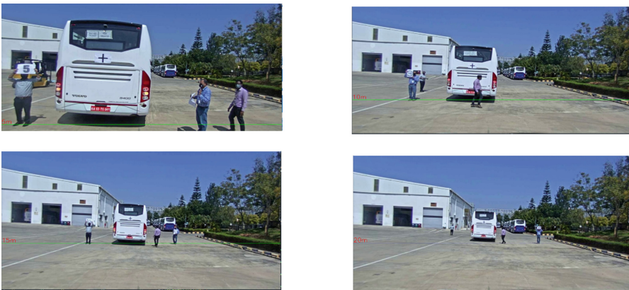
Fig. 5. Distance guidelines 5m(top-left), 10m(top-right),15m (bottom-left), 20m (bottom-right)
