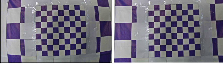
Fig. 2. 9*9 distorted image(left), 9*9 undistorted image (right)
