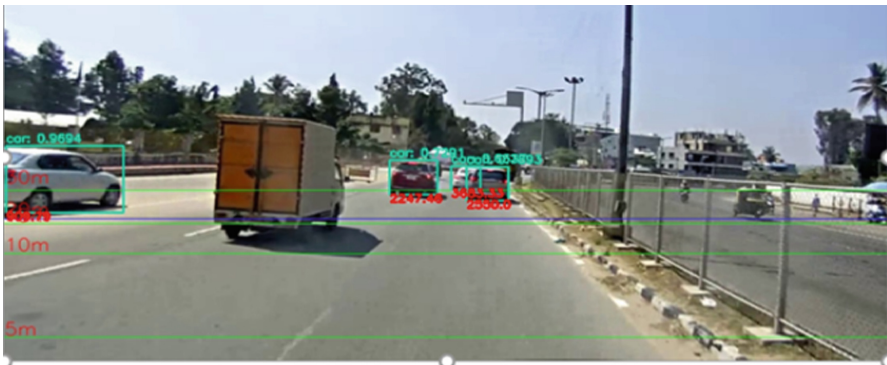
Fig. 9. Car detection result(YOLOv3)
