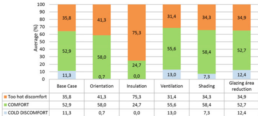
Fig. 5 Bar graph with percentage of hours in comfort and discomfort, and table with averages of temperature in comfort, heat and cold discomfort
