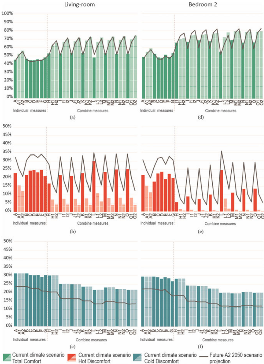
Fig. 2 Percentage of time in comfort or discomfort by case study, Current and future A2 2050 climate scenario, Living room: a Total time in comfort, b Time in discomfort due to heat, c Time in discomfort due to cold, Bedroom 2: d Total time in comfort, e Time in discomfort due to heat, f Time in discomfort due to cold
