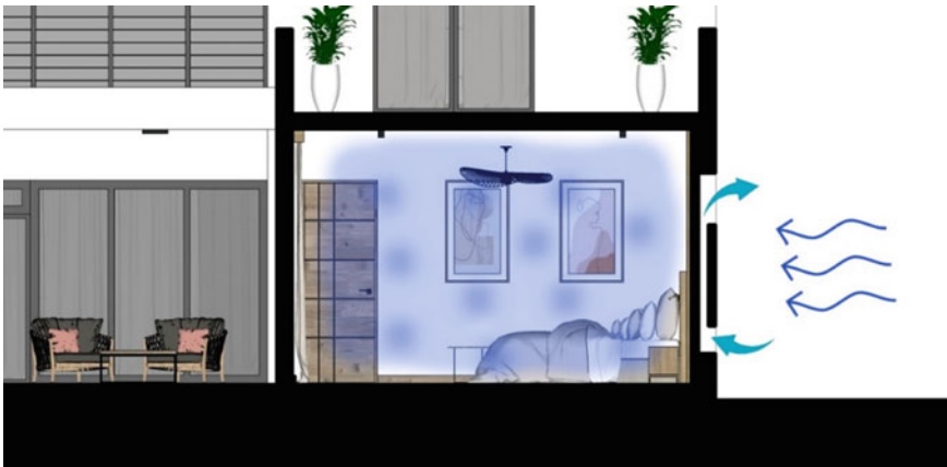
Fig. 7 Heat control with ventilated cavity
