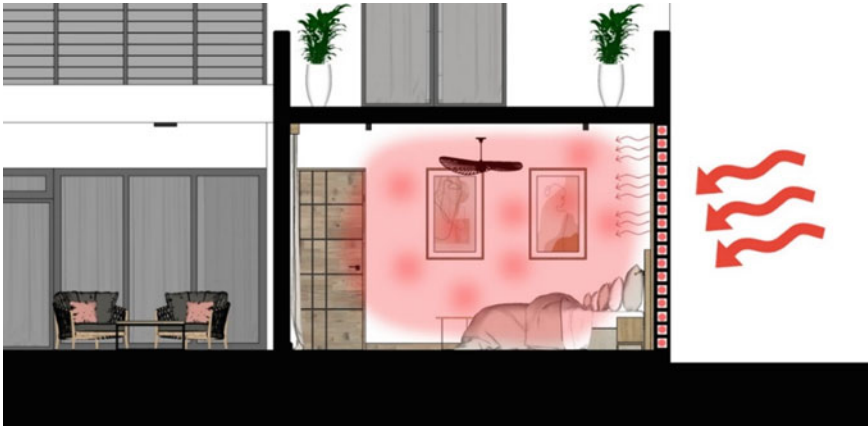
Fig. 6 Heat trapped in cavities with normal blocks
