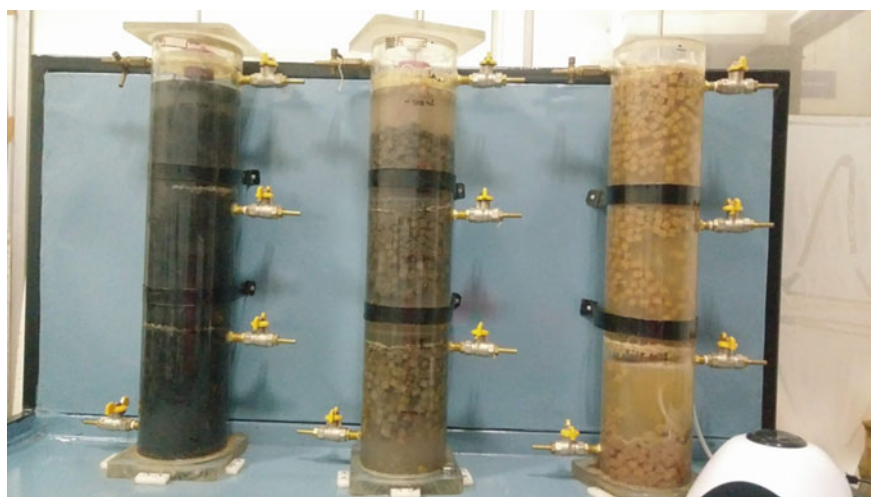
Fig. 1 Lab scale MBBRs with Polyurethane cubes as biofilm carrier media
