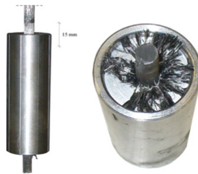
Fig. 9. Residues of fibers accumulated near the end of the anchorage, after cable's slip.
