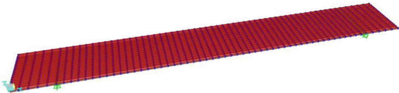
Fig. 2. FE model of the laboratory slab
