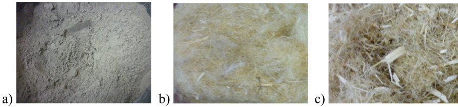
Fig. 1. Fly ashes (a), different type of natural (not treated) hemp fibers (b) and (c).
