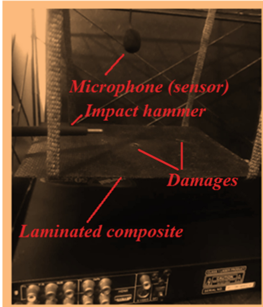
Fig. 7. Deploying the rectangular laminated composite plate, microphone, impact hammer, and boundary conditions.
