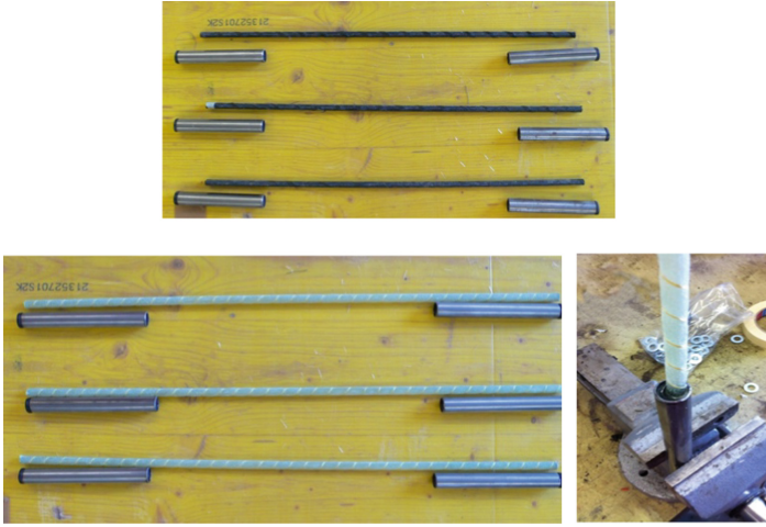
Fig. 1. Manufacturing of GFRP and CFRP rods samples.
