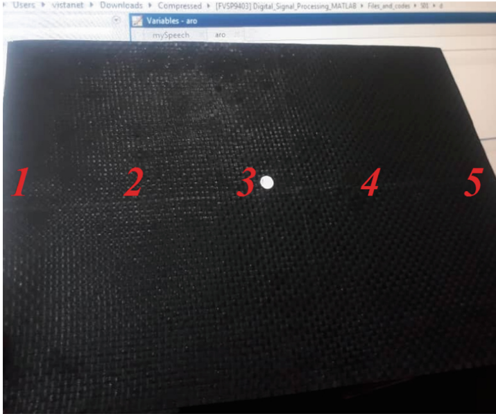
Fig. 8. Five points specified on the rectangular laminated composite plate as impact locations for Scenario 1.
