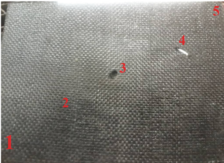
Fig. 19. Five points specified on the rectangular laminated composite plate as impact locations for Scenario 4.
