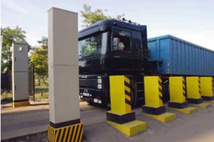
Fig. 3.19 Neuport and NeuTruck portal detection systems разработанные на основе ZnS/6LiF BC-704 detector. (Reprinted from http://www.crystals.saintgobain.com )
