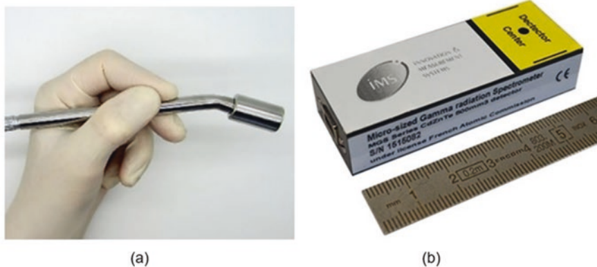
Fig. 5.5 (a) An example of a miniaturized probe used for radioguided surgery. SGDP Medical probe with planar detector with volume 0.25 \text{ cm}^3 developed by ZRF RITEC SIA ( http://www.ritec.lv/ ). (b) Micro-sized Gamma Spectrometer (The MGS series), fully integrated instrument based on a CdZnTe (CZT) crystal ( 0.06 or 0.5 \text{ cm}^3 ) operated at room temperature from IMS Innovation & Measurement Systems. ( https://www.imsrad.com/CdZnTe-spectrometers.php )
