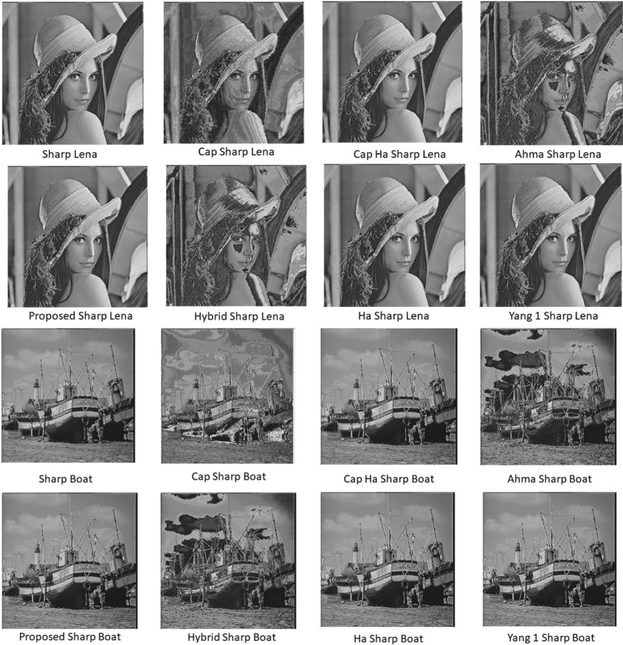
Fig. 16. Sharpening of image using different multipliers (First two rows sharpening of lena and the last two rows sharpening of boat; first image in row1 and row3 are the results using an exact multiplier).
