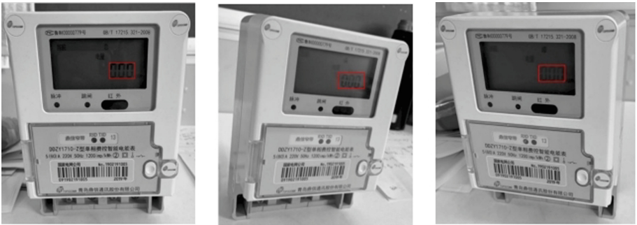
Fig. 6. Processed grayscale image and detection frame
