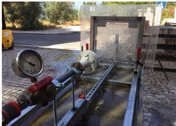
Fig. 3.3 Example of a spray test equipment (without sample) to assess earth products durability to water
