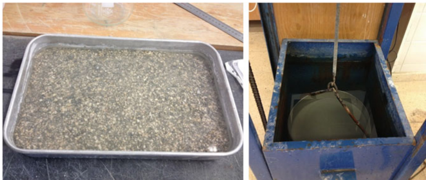
Fig. 4.1 Left: Sample immersed in sodium hexametaphosphate solution; right: Submersion of the set (sample, sieves, and support) for hydrostatic weighing
