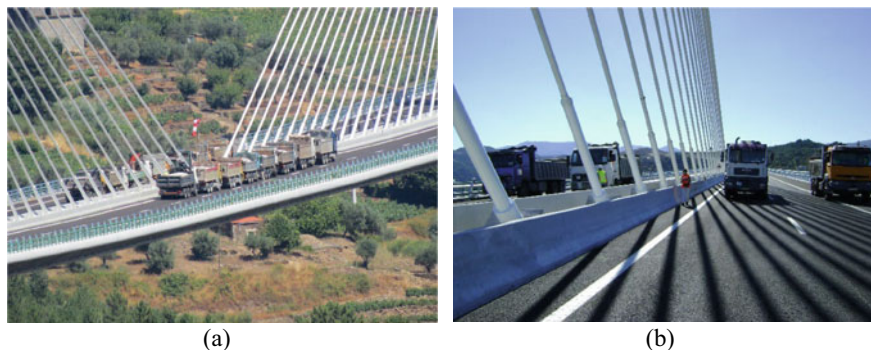
Fig. 10.4 Position of the vehicles during the test: a load case LC14 using 16 vehicles; b 4 vehicles side-by-side crossing the bridge to obtain the influence lines
