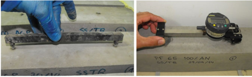
Fig. 4.2 Total shrinkage test
