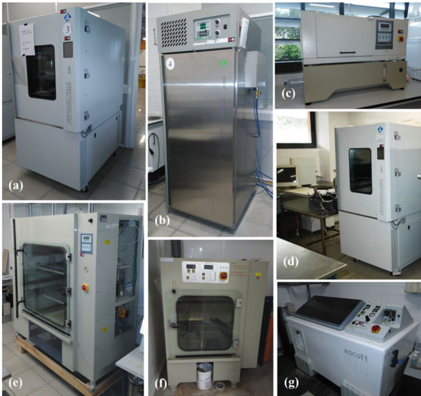
Fig. 2.4 Test chambers for accelerated durability tests: a Climatic; b Carbonation; c Xenon Arc; d Freeze–Thaw; e Corrosion; f SO 2 corrosion; g Salt fog
