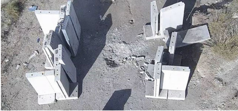
Fig. 9.12 Post Blast result of protected (left) and unprotected (right) T-Walls
