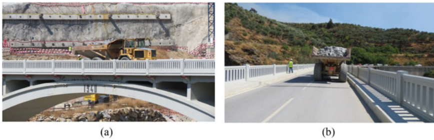
Fig. 10.18 Load test: a general view of vehicle crossing the bridge; b vehicle crossing at the downstream side of the traffic lane
