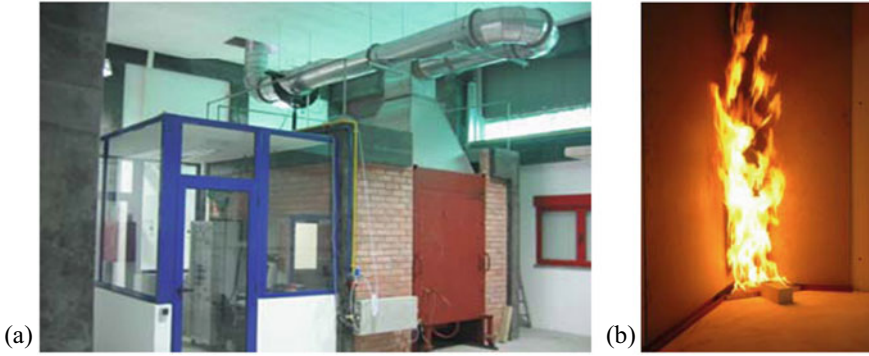
Fig. 16.2 a, b Insulated burning object (OIC/SBI), EN 13823, [5]
