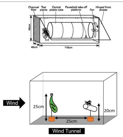
**Fig. 1.11** Wind tunnels. Upper panel: Design of the wind tunnel used by Grasswitz and Paine (1993) to study the behaviour of *Lysiphlebus testaceipes* (Hymenoptera: Braconidae), a parasitoid of aphids. The main (rectangular) chamber was constructed of Plexiglass, and the central (cylindrical) test section was constructed of Mylar (biaxially-oriented polyethylene terephthalate). Lower panel: Schematic diagram of the wind tunnel used by
