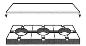
**Fig. 1.9** The static-air olfactometer of Vet (1983). The apparatus comprises three Perspex blocks glued together and covered by a single glass lid (a single Perspex block would also suffice, although it may be more difficult to excavate). The excavations (chambers) in the blocks are connected by corridors. The chambers, measured internally, are 50 mm wide and 16 mm deep; the corridors are 10 mm wide and 5 mm deep. Reproduced by permission of E.J. Brill (Publishers) Ltd
