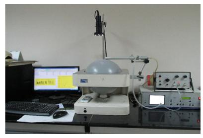
**Fig. 1.10** A locomotion compensator being used to test the responses of host larvae to plant volatiles (photograph K. S. Shameer). Examples of parasitoid walking tracks can be found in Vet and Papaj (1992)
