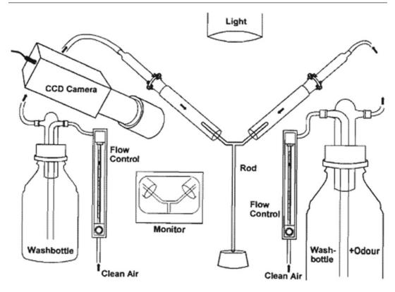
**Fig. 1.7** Open Y-track olfactometer. The insect is placed on the base of the vertical rod and starts walking upward. At the junction it will choose between a clean air flow, here at the left, and an air flow loaded with plant odour,
