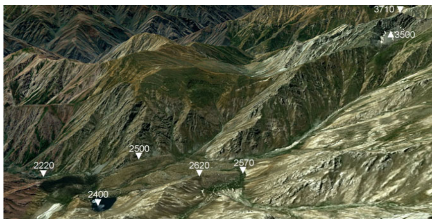
Fig. 3.7 The Aigyrkul rock avalanche in the Tupolangdaria River basin. The source zone is at the top right of the image between elevation marks 3,710 and 3,500 m a.s.l. Rock avalanche deposits stretch from 2,570 to 2,220 m a.s.l. (after Strom and Abdrakhmatov 2018. Reprinted with permission of Elsevier)
