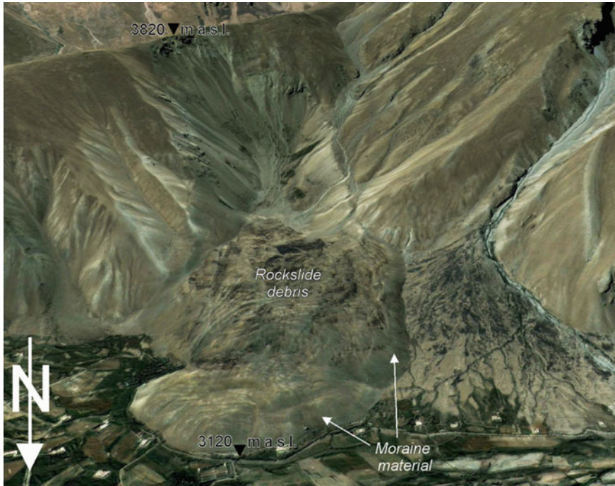
Fig. 3.10 Oblique view of the Imom rock avalanche. The inner part of its body is composed of crushed crystalline rocks, while the outer part is by the bulldozed moraine material
