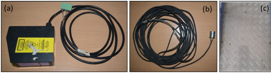
Fig. 10.5 Sensors installed on the flow path and the deposition zone a laser sensor for measuring flow height b pore water pressure sensor c the rough surface of the flow path
