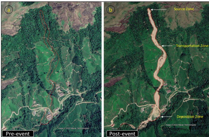
Fig. 10.1 Source zone, transportation zone and deposition zone of a typical debris flow a pre-event b post-event image of Pettimudi debris flow at Idukki district, Kerala State, India (Source Google Earth)
