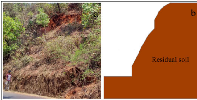
Fig. 8.3 Pictorial representation of soil slope a Field photograph of the slope and b general illustration for slope stability analysis
