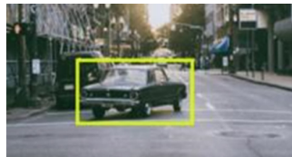
Fig. 13. YOLO uses a single bounding box regression for the purpose of object detection and classification. Confidence score signifies what the likelihood of the bounding box containing a particular object.
