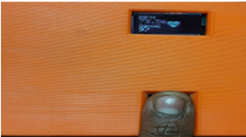
Fig. 3. Developed IoT-based pulse oximeter showing SpO 2 and heart rate values.
