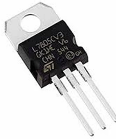
Fig. 6. LM7805 voltage regulator
