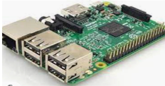
Fig. 3. Raspberry Pi 3 board with two USB ports
