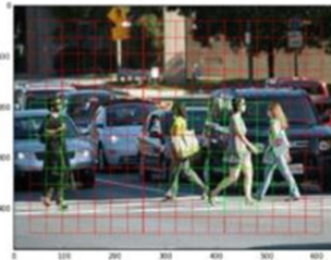
Fig. 12. The passing input image that is fed to the neural network is split into grid cells of equal dimensions.
