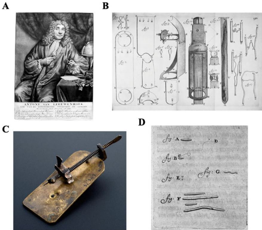
Fig. 1 Illustrations from the works of Antonius van Leeuwenhoek, one of the world’s first microscopists to examine the details of unicellular life. (a) Portrait of van Leeuwenhoek holding his simple microscope. From Antonius van Leeuwenhoek. Mezzotint by J. Verkolje, 1686. Public Domain Mark. Wellcome Collection. (b) An illustration on the design of van Leeuwenhoek’s single-lens microscopes by Henry Baker. From Arcana naturae detecta / Ab Antonio van Leeuwenhoek, 1695 . Wellcome Collection. (c) A replica of van Leeuwenhoek’s simple microscope. From Leeuwenhoek simple microscope (copy) , Leyden, 1901–1930. Science Museum, London. Wellcome Collection. (d) Drawings from van Leeuwenhoek’s notes, depicting the size, shape, and movement of bacteria in a dental plaque sample observed under the microscope. From Arcana naturae detecta/Ab Antonio van Leeuwenhoek . (b, c, d) Reproduced with permission under CC-BY-4.0 licence ( https://creativecommons.org/licenses/by/4.0/ ). Credit: Wellcome Collection
