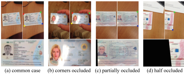
Fig. 5. Examples of occluded points prediction. Each case contains three images, namely, the input image (top left), the predicted corners on the input image (top right), the localized document after removing the perspective transformation (bottom).
