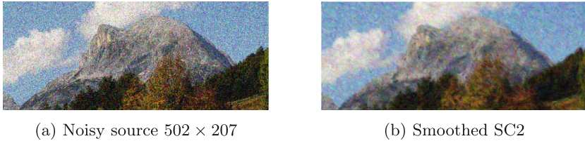
Fig. 14. Denoising of a colour image with Gaussian noise. (a) Image HoheMunde40 degraded by Gaussian noise ( \sigma = 40 ). – (b) Denoised by applying AMSS smoothing with SC2 to the 206 842 level lines. (Image source: https://www.telfs.at/files/user_upload/915x375/wohnen-leben-hohe-munde-hausberg-telfs-02.jpg , accessed: 2022-02-02.)
