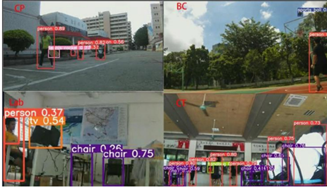
Fig. 7. Object detection results on YOLOv5 for moving + dataset.
