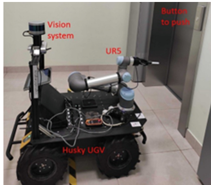
Fig. 1. Setup for an example task of robotic button pushing.
