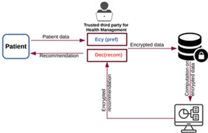
Fig. 4 Privacy enabled healthcare recommender system with homomorphic encryption
