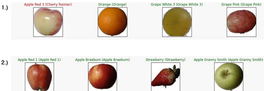
Fig. 4. Predictor model results (green if predicted = true label) 1.) CNN and 2.) ResNet50 V2 (Color figure online)
