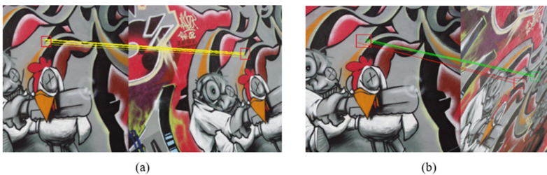
Fig. 1. The effect of the GMS algorithm on the affine transformation images. In Fig. 1(a), when the degree of affine transformation is small, the GMS filtered features are matched accurately, as shown in the grid area boxed in red; however, in Fig. 1(b), when the degree of affine transformation is large, the GMS algorithm assumes that the green grid is the correct counterpart, but the actual correct counterpart is the red grid. (Color figure online)
