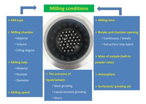
**Fig. 3** Most commonly changed experimental conditions during high-energy milling. (Reprinted by permission from Springer Nature Customer Service Centre GmbH: Springer Nature [5] [COPYRIGHT] (2021))
