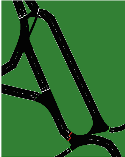
Fig. 2. SUMO network converted from OpenStreetMap: before corrections.
