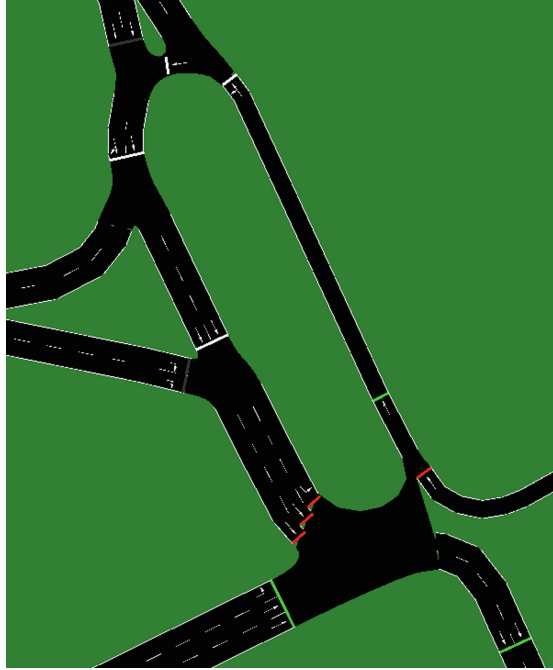
Fig. 3. SUMO network converted from OpenStreetMap: after corrections.
