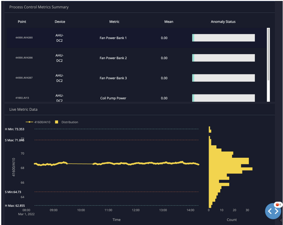
Fig. 5. Lower panels of the data center anomaly detection dashboard. The upper panel shows a table of metrics associated with a selected device, with columns indicating the label of the point in the streaming database, the name of the associated device, a short description of the metric, the mean value over the past six hours, and the current anomaly status shown as a bar progressing from green (OK) to red (high alert). The lower panel shows a time-series of the selected point over the past six hours with points exceeding the anomaly thresholds highlighted in red. The soft and hard anomaly shown as red dashed and solid lines. (Color figure online)
