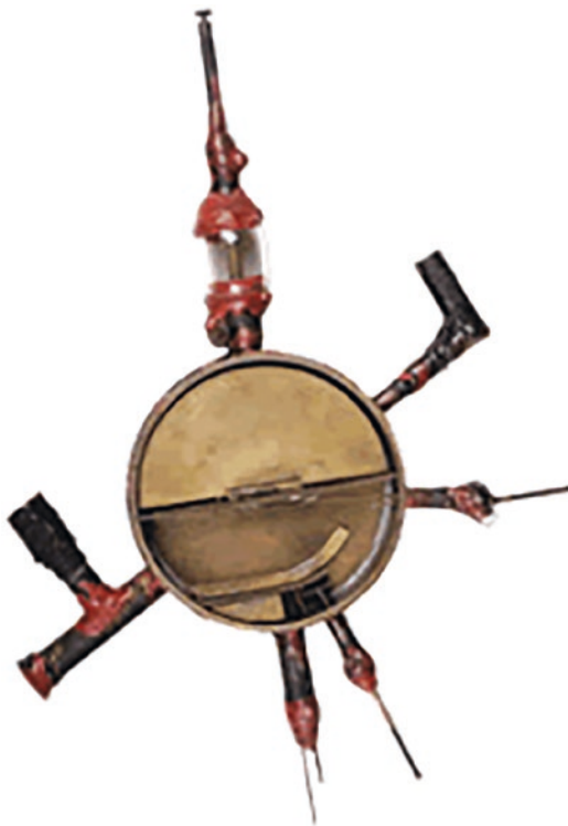
Fig. 8.5 The first working model of a 4.5 in. cyclotron, which accelerated protons to 80 KeV energy [11]
