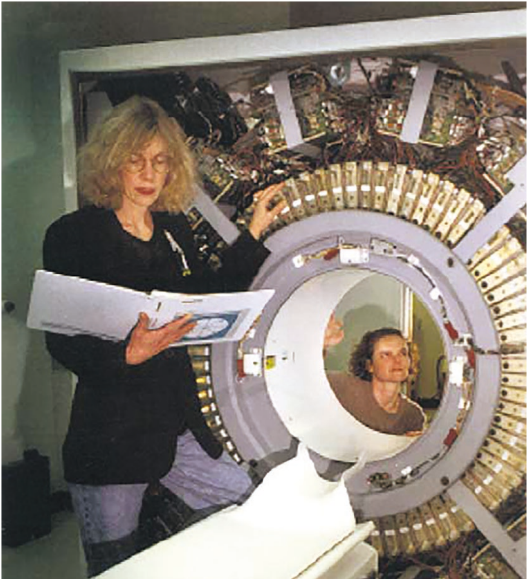
Fig. 5.8 The typical PET scanner with ring detector configuration
