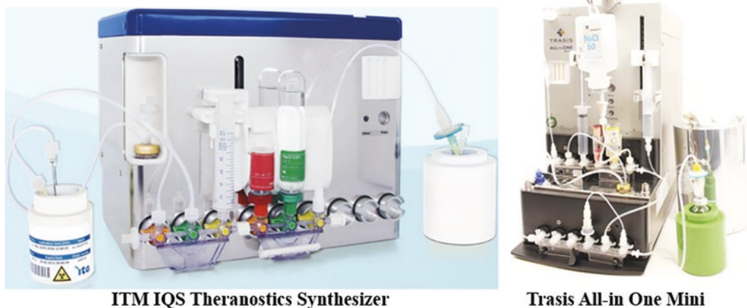
Fig. 12.8 Examples of automated synthesis modules for the labeling of metal radiopharmaceuticals
