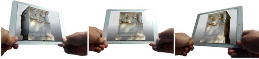
Fig. 2 Interactive visual inspection of a 3D digitised inscription along with the inscription bearer. The user can view the object from different perspectives using natural motions
