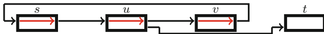
Fig. 1. Illustration of a consecutive circuit, with four vertices \{s, u, v, t\} and three mandatory transitions \Pi = \{ \langle s, u, v \rangle, \langle u, v, s \rangle, \langle v, s, u \rangle \} .
