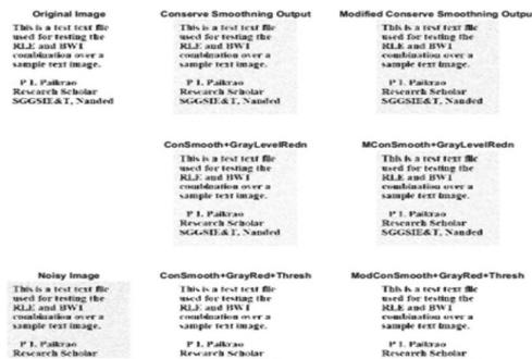
Fig. 8. The result of combining smoothing, grey level reduction and thresholding
