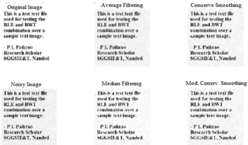
Fig. 5. Result of various smoothing algorithms
