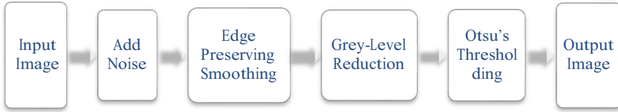
Fig. 4. Flow of proposed scheme for document image enhancement
