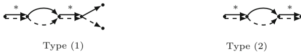
Fig. 3. Accident-1 manageable graphs for two messages. The solid and dashed lines correspond to edges in \mathcal{W}_i and \mathcal{W}_j , respectively. * denotes optional parts in the walk.
