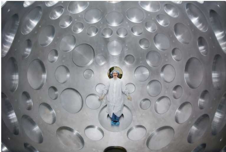
Fig. 8.12 The interior region of a target chamber of an ICF facility; notice the large diameter. (Image courtesy of Mr. Eugene Kowaluk, Laboratory for Laser Energetics, University of Rochester)
