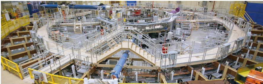
Fig. 8.22 A recent photograph of the Sandia Z-Machine. The technology for this machine evolved from many earlier facilities centered on using beams of particles to start ICF events. These machines can trace their lineage back to the work of Sandia researcher Gerold Yonas in 1970 [14]. Sandia built or planned for several of these machines, including Hydra, Proto I, Proto II, the Electronic Beam Fusion Accelerator (EPFA I and II), the Particle Beam Fusion Accelerator (PBFA-I and II) and Saturn. (Image permissions from Troy Rummier of Sandia National Laboratory)
