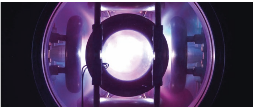
Fig. 2.11 The polywell has plasma-facing magnets. The surface of these magnets is designed to be ultrasmooth to minimize plasma conduction. Its design keeps the magnetic field lines from running into surfaces and thus maintains a space between the plasma and the magnets. Over time, these magnets would crack and swell under the neutron load. (Image credit: Dr. Jaeyoung Park)
