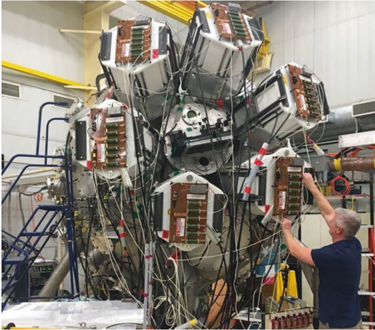
Fig. 9.15 The Plasma Liner Experiment under construction at Los Alamos National Laboratory on January 31, 2017 [2]. Note the plasma cannons, which are the attached knobby and bulky hexagonal white blocks. (Image approval by Los Alamos (LA-UR-22-24212))
