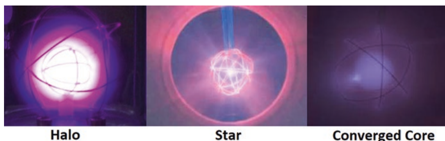
Fig. 10.6 The three modes of fusor operation as determined by Dr. Tim Thorsen at the University of Wisconsin-Madison. (Image source: Wikipedia)
