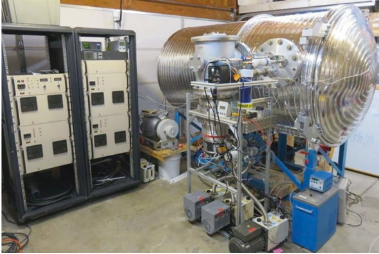
Fig. 6.18 Horne Technologies superconducting device built in Boulder, Colorado, in 2020. This machine used ReBCO superconductors to run for over 20 min at fields of 1.5 teslas. Image courtesy of Horne Technologies
