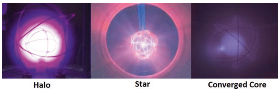
Fig. 2.2 The three modes of a fusor. On the left is the “halo mode,” which is characterized by a broad glowing cloud of plasma and gas. In the center is the “star mode,” which looks like a shining star. In the “converged core” on the right, gas pressure is so low that the glowing effect is very weak. Changing the gas pressure inside the fusor results in causes switching between these three modes of operation. The star mode gives you the most fusion reactions, though, as discussed later, fusors will never lead to net power
