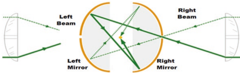
Fig. 8.5 A schematic showing how the double-bounce illumination system worked. Beams would pass through pinholes into a mirror chamber. Those beams would reflect and strike a pellet of DT fusion fuel from different directions, compressing it to ignite fusion. (Image source: Wikipedia)
