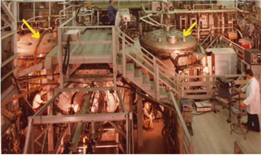
Fig. 4.8 A 1978 photo of the LLNL laboratory, which housed the 2X and baseball mirror machines. The end coils were housed in large vacuum chambers that look like big stove pots on either end of the laboratory (yellow arrows). The plasma oscillated between these. (Photo credit: Lawrence Livermore National Laboratory)
