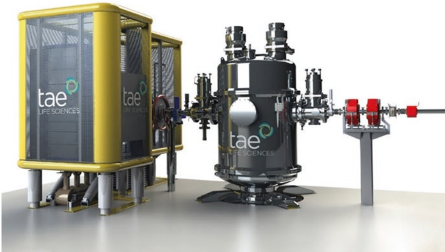
Fig. 2.17 A CAD model of boron neutron capture therapy machine now being developed by TAE Life Sciences
