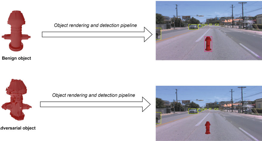
Fig. 1. Attack goal is to create an adversarial object that is invisible to camera model
