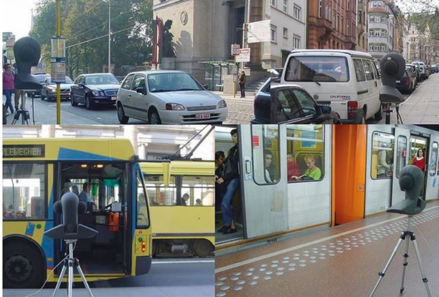
Fig. 6.4 Examples of recording sites using artificial heads in different acoustic environments. All sites are public areas with different forms of transportation noise
