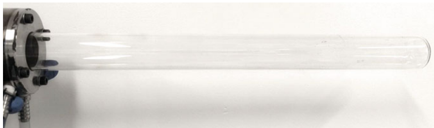
Fig. 1 Vacuum reactor tube connected to a steel cooling collar
