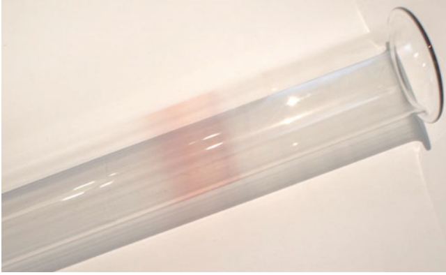
Fig. 3 Na deposition band formed from the sublimation of LMS-1 at \sim 1150\text{ }^{\circ}\text{C} for 8.8 h at 3.83\text{E-}08 atm, after pre-processing for 3.5 h at similar conditions
