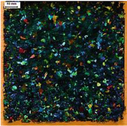
Fig. 4 View of samples manufactured by hot-pressing: (a) K2 composite, (b) K3 composite
