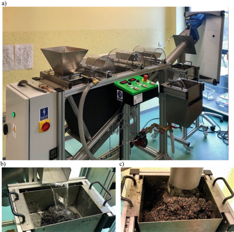
Fig. 2 View of the flotation and sedimentation device for separation process: (a) flotation tank, (b) separated light fraction, and (c) separated heavy fraction
