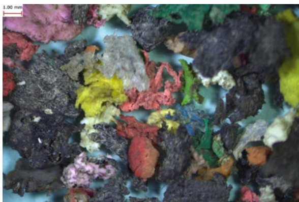
Fig. 1 Mixture of polymeric cable wastes introduced into the flotation process
