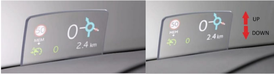
Fig. 5 Citroën HUD – sliding screen and height setting
