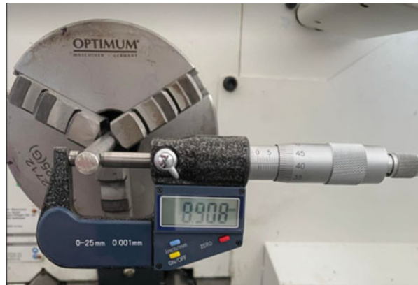
Fig. 7 Measuring of the diameter deviation by ((a) LTS, (b) CS)
