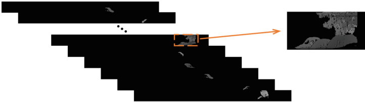
Fig. 4. After BEV preliminary segmentation, we project each clustered point cloud to a range image separately. The pixel brightness represents the range value of the points. Pure black pixels means no point or the point out of the region.
