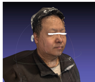
Fig. 6. 3D face reconstruction result after post-processing with Poisson surface reconstruction.
