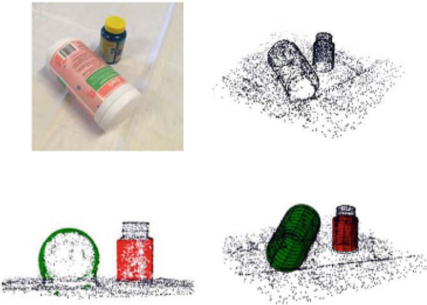
Fig. 2 3D recovery of circular cylinders. Top-left: one of the 22 images in 2D. Top-right: the 6500 points recovered in 3D. Bottom left and right: The 2262 inlier points viewed in two different angles. Images partially © 2021 IEEE. Reprinted, with permission, from Yang et al. (2021)
