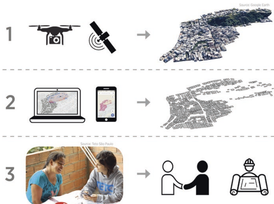
Fig. 12.2 Teto's mapping process, step-by-step: (1) acquiring drone or satellite imagery; (2) digitizing building footprints, with on-site verifications using Google My Maps; (3) validating GI data to obtain geographic information that may support upgrading projects. Elaborated by the authors, based on Google Earth (2018) and Pessoa Colombo (2019)
