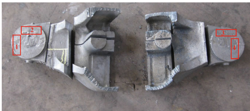
Fig. 11 The casting component used for the measurements of mechanical properties
