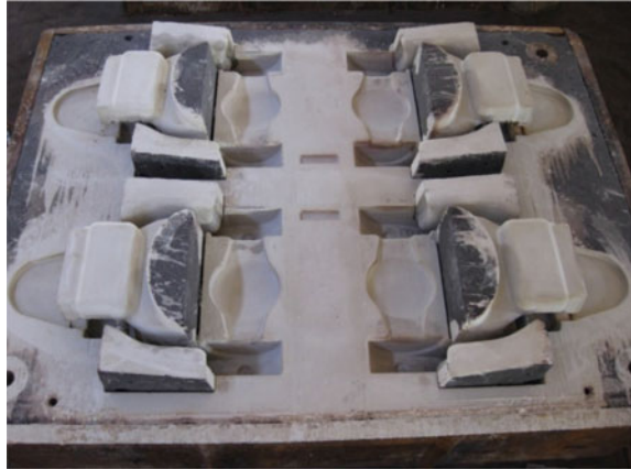
Fig. 9 One of the lower casting mold with the cores
