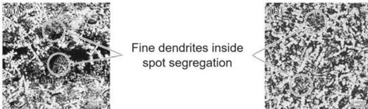
Fig. 5 Fine dendrites inside spot segregation in central area on longitudinal section of billets No. 1 (a) and No. 2 (b)
