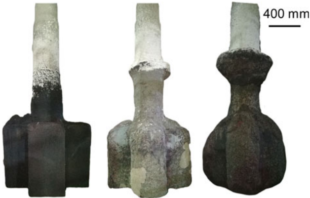
Fig. 2 Morphology of the same impeller with the initial state (left), after employed 120 heats (middle), and after employed 220 heats (right)
