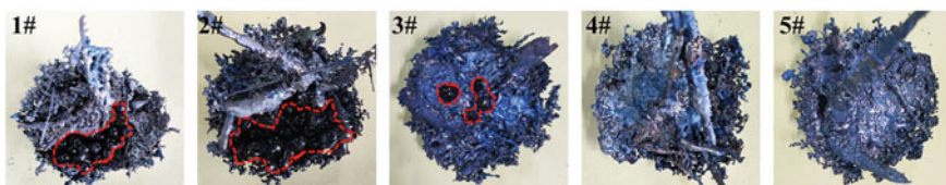
Fig. 5 Morphology of droplets formed under different atmospheres
