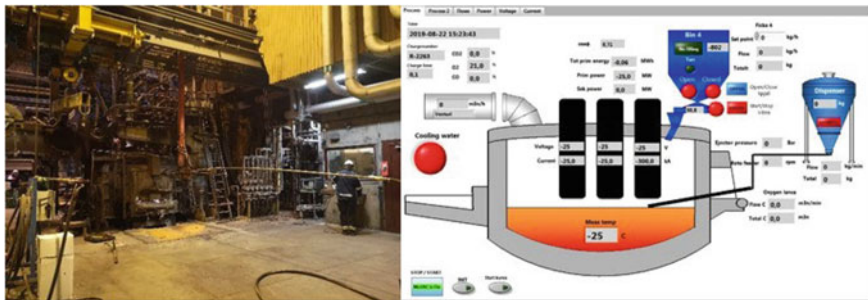
Fig. 3 Swerim's pilot EAF furnace, the layout (left) and the control system (right)
